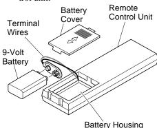
Figure 50 - Installing Battery in Hand-Held Remote Control Unit
